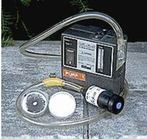
Example of a personal sampling pump with a 25 mm MCE filter used to monitor air quality during asbestos abatement projects.
