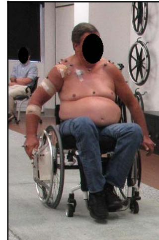
Figure 1. A subject wheeling on a carpeted level floor using the IntelliWheels geared manual wheelchair wheels.
