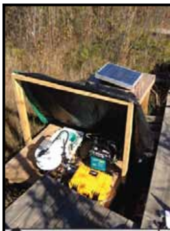
Field installation of the LI-COR 8100A automated soil gas flux analyzer
