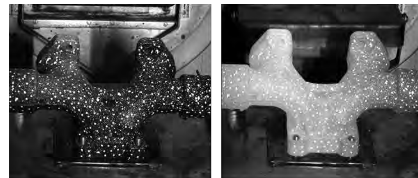
Fig. 5 High Temperature DIC, left is filtered with blue light, right is unfiltered light [3].
